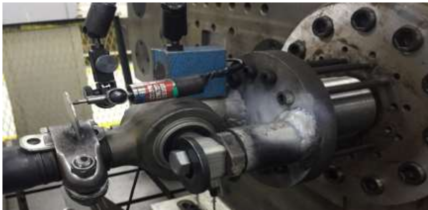
Figure 5. Test Setup for Radial Stiffness
