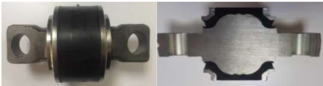
Figure 3. Torque Rod Bushing (Left) and Its Cutaway View (Right)
