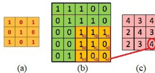
Fig. 1. Convolution operation (a) filter, (b) matrix of the image, (c) convolution result [22]
