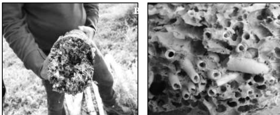
Figure 4. Damage caused by shipworms at wooden poles used in fixed off-bottom cultures of Gracilaria gracilis (A) and tunnels occupied by calcareous tubes of shipworms (B).
