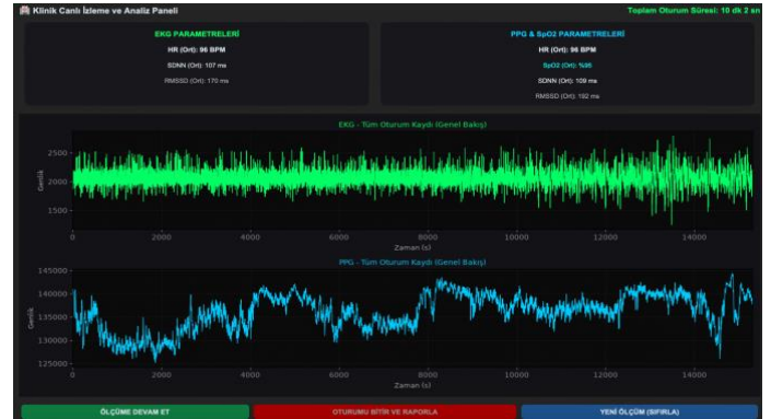
Figure 3. Real time clinical monitoring and analysis dashboard after a 10 min 2 s resting session. The upper panels show mean HR, SDNN and RMSSD for ECG (left) and PPG + SpO 2 (right). The lower panels display the complete ECG (green) and PPG (blue) waveforms recorded during the entire session.
