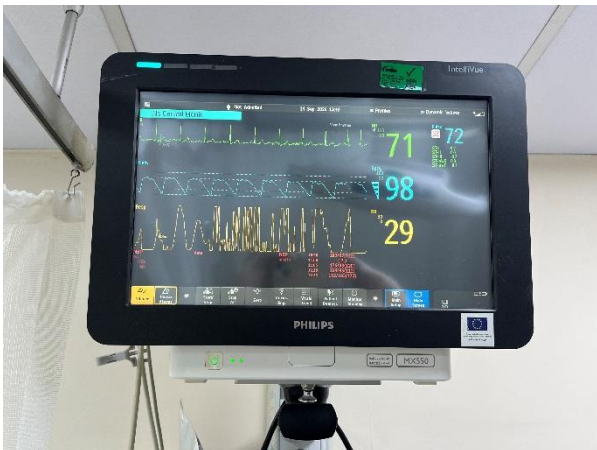
Figure 2. Clinical grade reference monitor (Philips IntelliVue MX550) present in the recording environment, showing concurrent heart rate and SpO 2 values for visual comparison.
