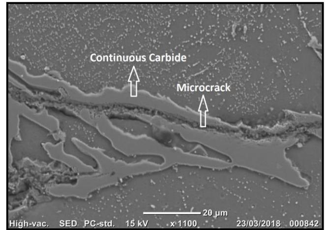
**Figure 17.** SEM image of microcrack
