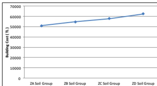
**Figure 9.** Construction Cost Graph of Structures of Different Local Site Classes.
