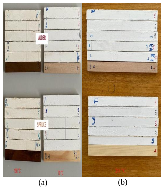
Figure 3. The samples' image after 70 °C and 150 °C of thermal aging process for 624 h (a) and at 20 °C (b)
