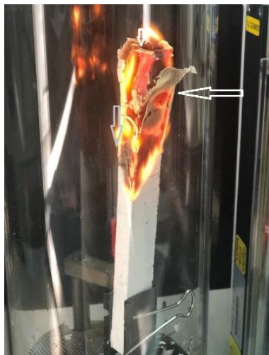
Figure 6. The LOI test sample on coated spruce (LT2)
