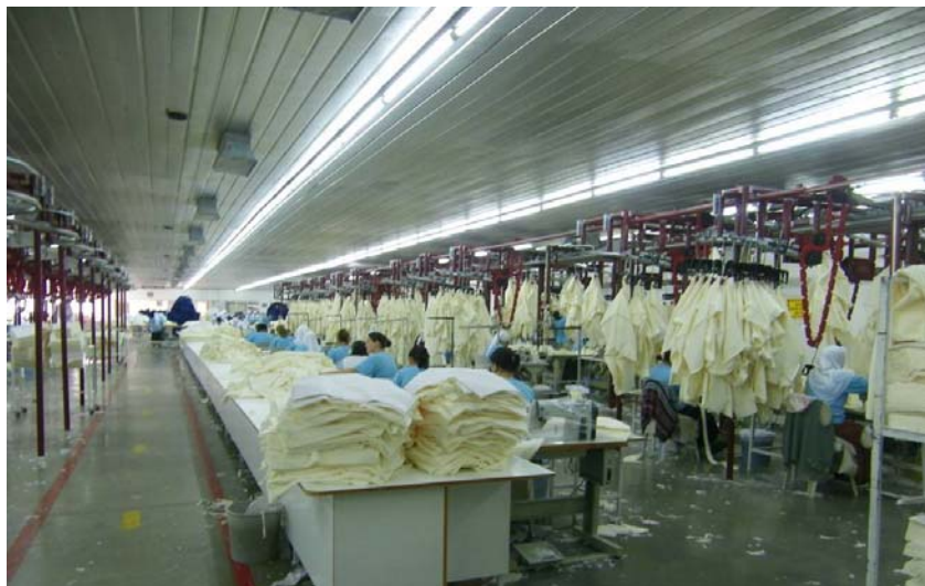
Figure 1. Preparation line (on the left) and assembly line with the overhead conveyer (on the right)
