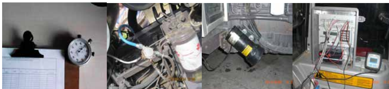
Figure 2. Time study table, fuel gauge, speed radar and data storage unit.
