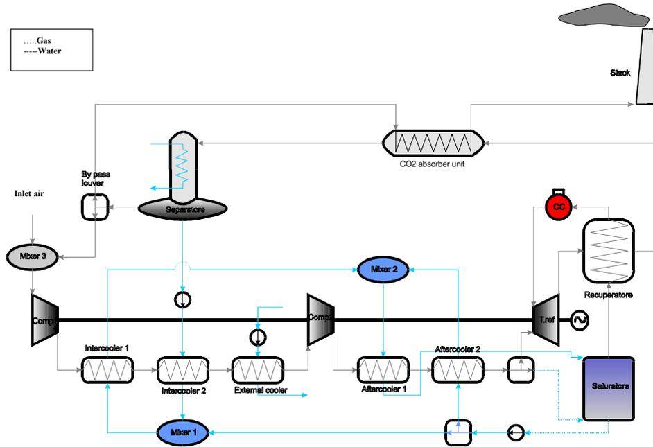
Figure 9. Schematic of the SC-HAT proposed power plant
