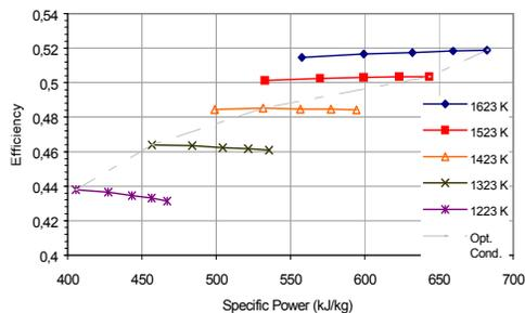
Figure 10. Expected performance of the basic SC-HAT cycle
