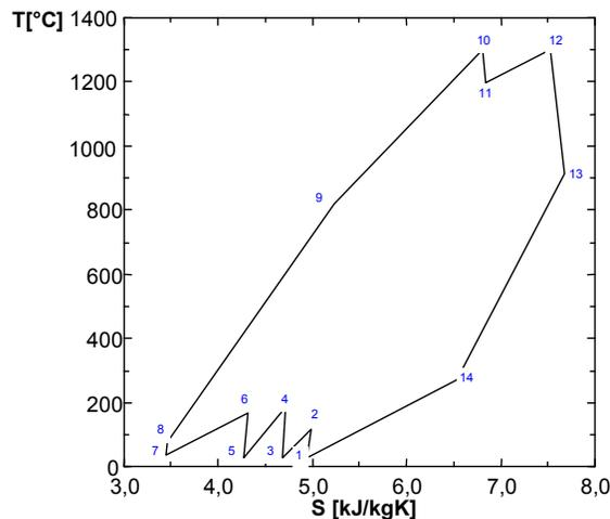
Figure 14. T-s diagram of the semiclosed cycle with liquid sequestration of CO<sub>2</sub>
