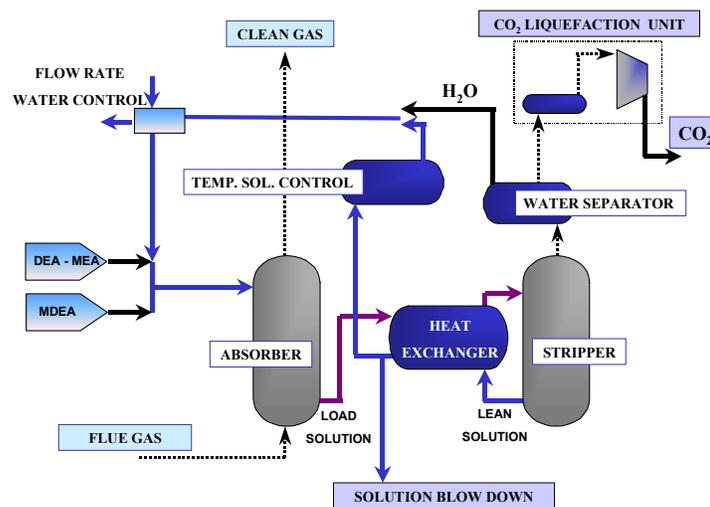
Figure 3. Schematic of the scrubbing system for CO<sub>2</sub> separation.
