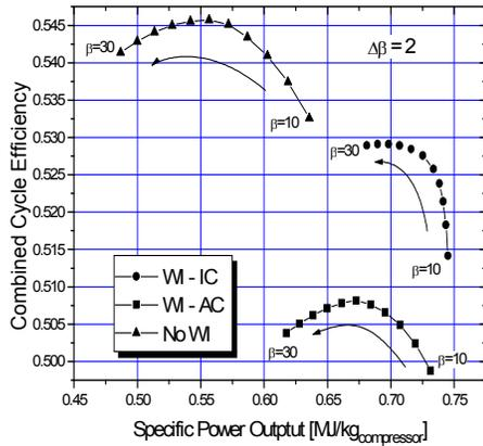
Figure 2. Performance map of the SCGY/CC cycle without and with reinjection of the recovered water (intercooled and aftercooled options).
