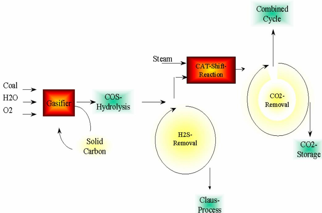
*Figure 12. Basic layout of the gasifier section of an IGCC power plant, showing location for pressurised chemical scrubbing of CO<sub>2</sub>*
