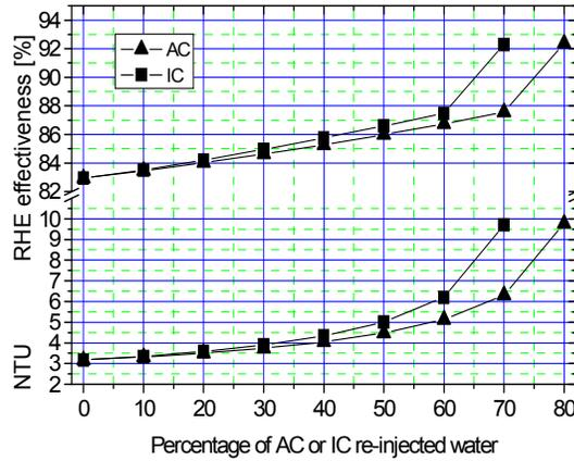
Figure 8. NTU and effectiveness of the regenerative heat exchanger. Sensitivity to level and mode of water injection. Hybrid CC/RE solution.
