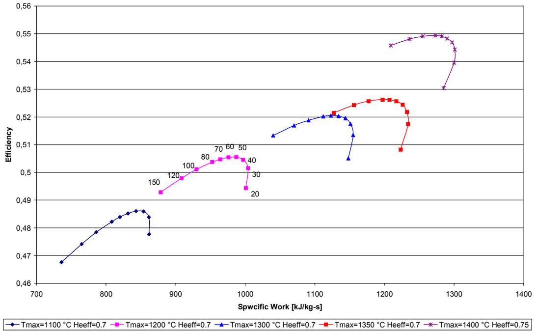
Figure 15. Performance map of F-Matiant cycle; sensitivity to max. firing temperature  $T_{10}$  and intermediate pressure  $p_{11}$ ;  $p_{max} = p_8 = 250$  bar; Heat exchanger effectiveness ( $HeEff$ ) = 0,75
