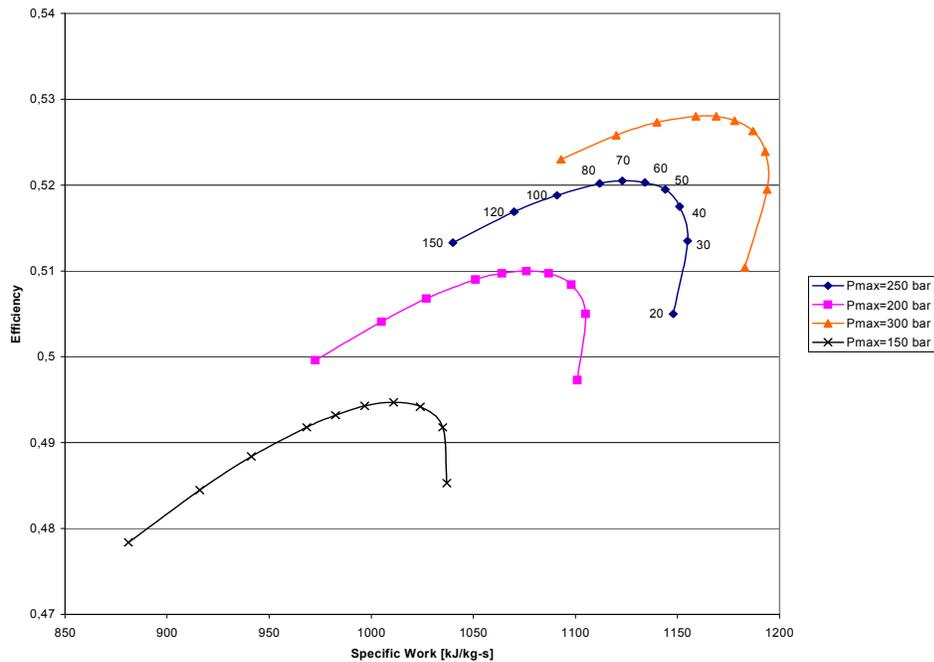
Figure 16. Performance map of F-Matiant cycle; sensitivity to max. cycle pressure  $p_{max} = p_8$  and intermediate pressure  $p_{11}$ ; firing temperature  $T_{10} = 1400$  K,  $HeEff = 0,75$ .
