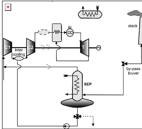
Figure 5. Schematic of the SCGT/RE cycle.
