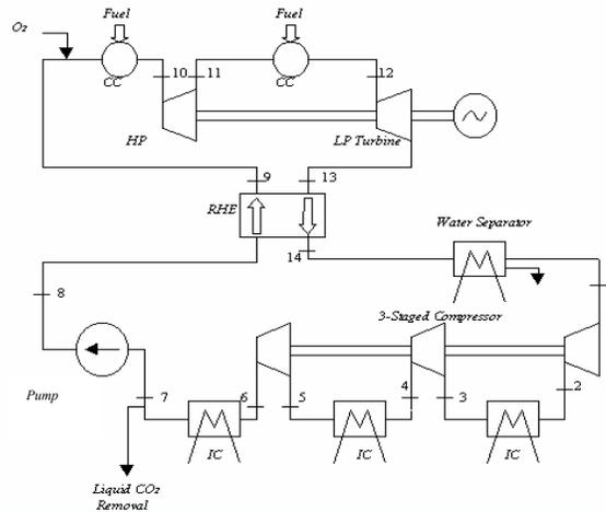
Figure 13. Layout of the semiclosed cycle with liquid sequestration of CO<sub>2</sub>
