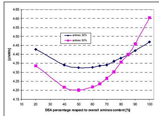
Figure 4. Additional cost (per unit energy of electricity) for CO<sub>2</sub> separation (SCGT system).
