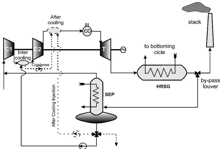
Figure 1. SCGT/CC power plant with compressor intercooling and aftercooling.
