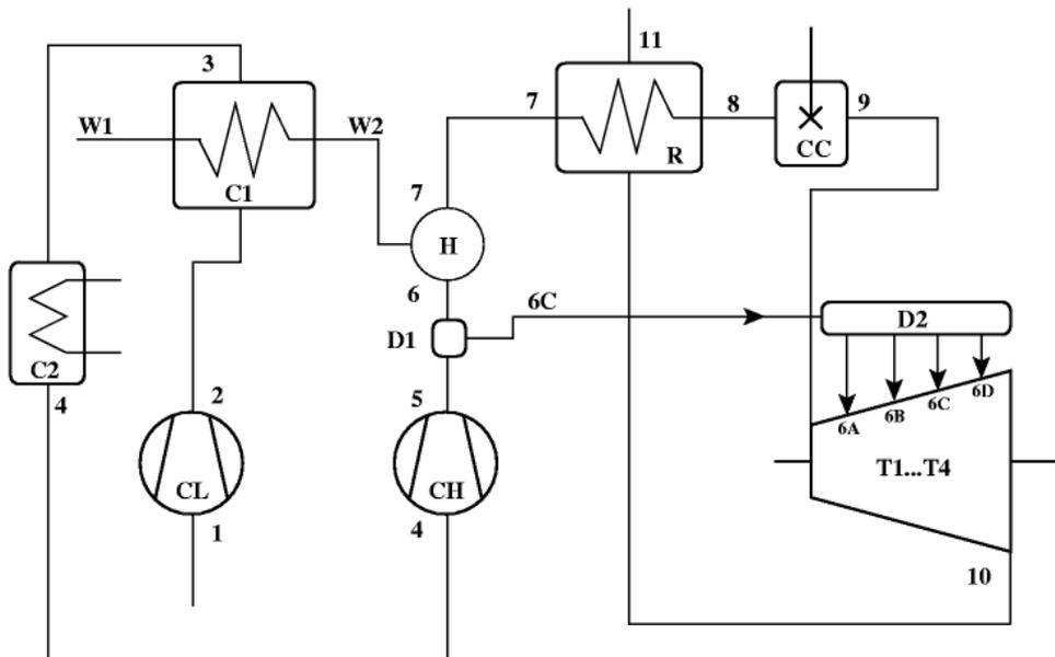
Figure 1. Scheme of the single-point water injection HAT power plant with cooling of turbine blades (CL, CH – low pressure and high pressure stage of the compressor, T1..T4 – stages of the turbine, C1 – interstage cooler and preheater of the injection water, C2 – external interstage cooler, CC – combustion chamber, H – humidifier of the compressed air, D – distributor of the cooling air, R – regenerative air preheater, 1...11 – streams of working fluid, W1, W2 – streams of the injection water).
