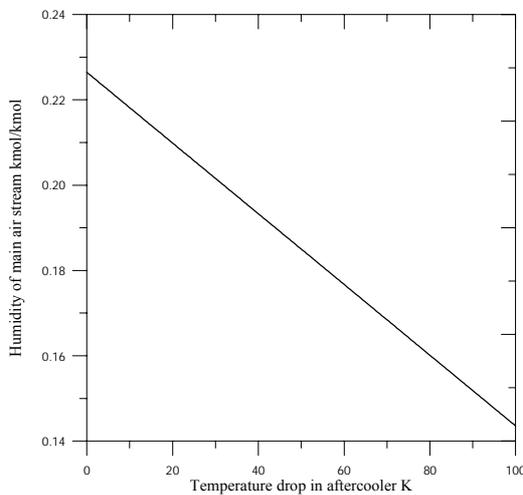
Figure 7. Influence of temperature drop in the after cooler on humidity of the main air stream
