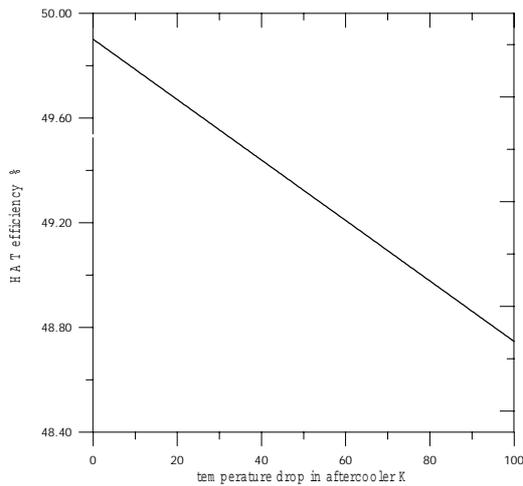
Figure 6. Influence of temperature drop in the after cooler on HAT turbine efficiency
