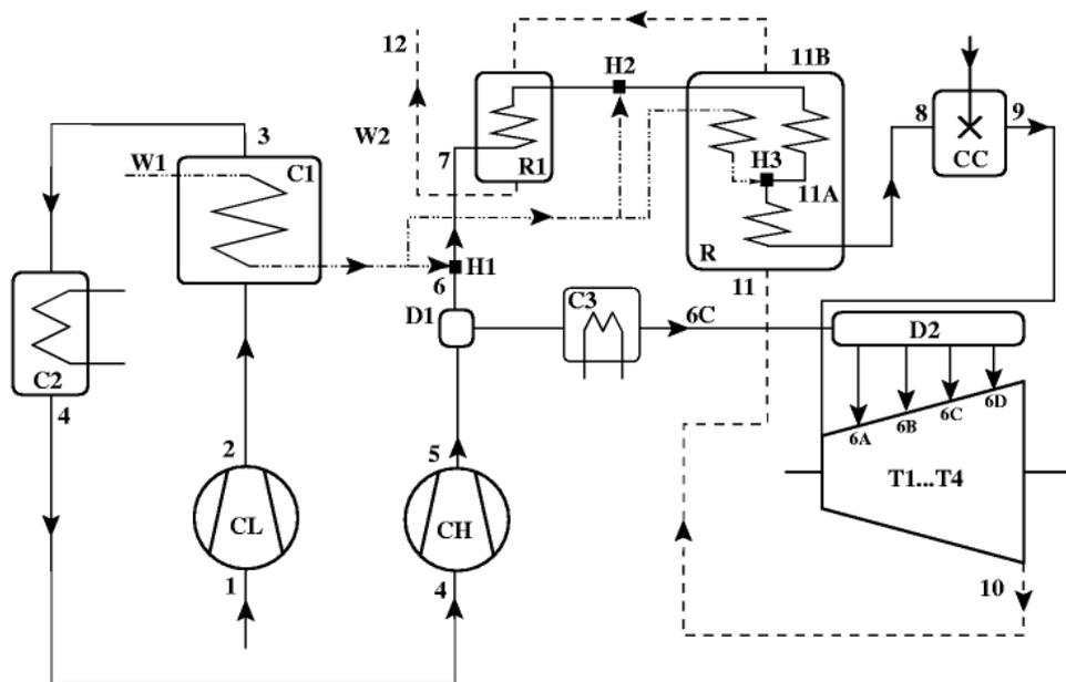
Figure 4. Scheme of the multi-point water injection HAT power plant with cooling of turbine blades with after cooler applied to the blades cooling air stream (C3 – after cooler, other symbol as in Figure 1)
