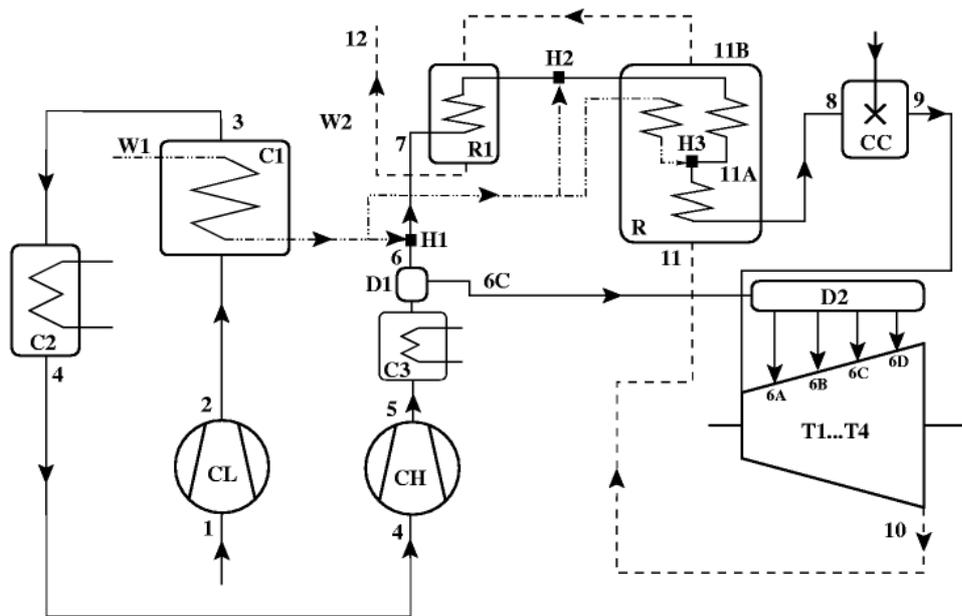
Figure 3. Scheme of the multi-point water injection HAT power plant with cooling of turbine blades with after cooler applied to the whole compressed air stream (C3 – after cooler, other symbol as in Figure 1)
