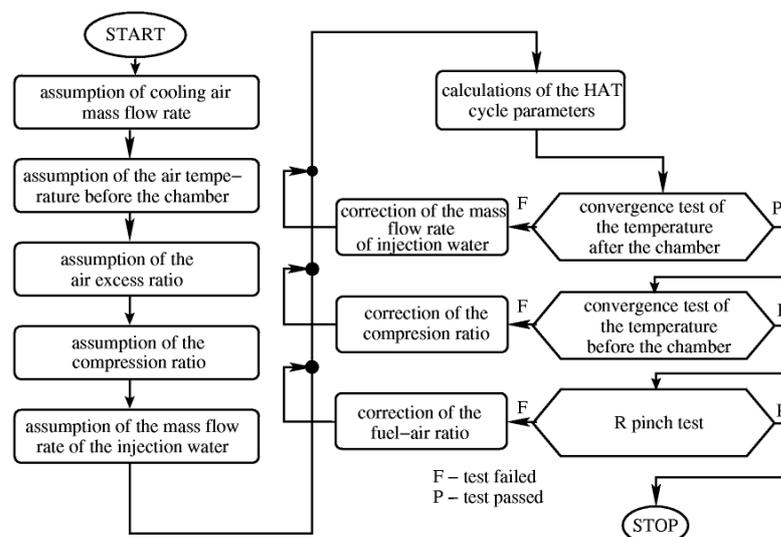
Figure 5. Block scheme of the calculations procedure. R pinch test denotes the test of minimal temperature difference in the regenerator (R in Figure 1)
