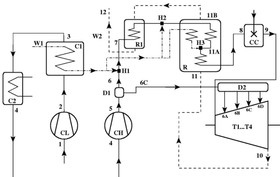
Figure 2. Scheme of the multi-point water injection HAT power plant with cooling of turbine blades (H1...H3 – stages of humidifier, other symbols as in Figure 1)
