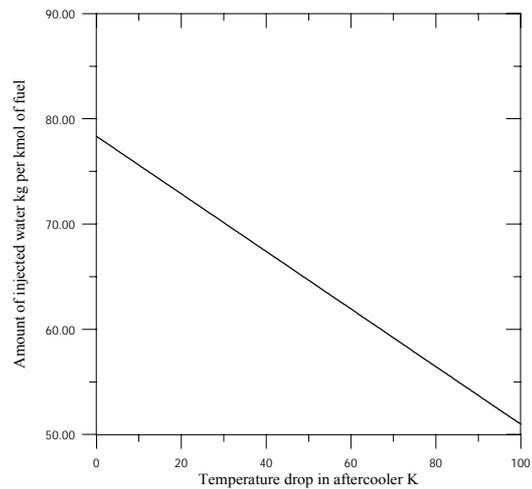
Figure 9. Influence of temperature drop in the after cooler on the amount of injected water
