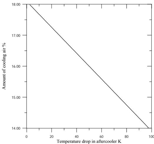
Figure 8. Influence of temperature drop in the after cooler on amount of the cooling air
