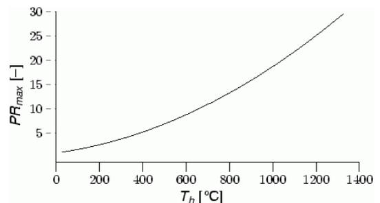
Figure 3. Upper limit of the pressure ratio for a gas turbine with recuperation ( $T_1 = 298$  K)
