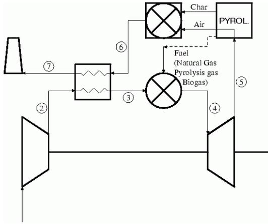
Figure 6. Flowsheet of an IFGT with supplementary firing
