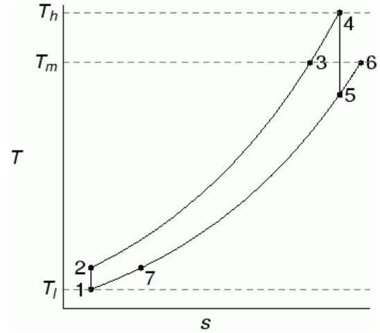
Figure 7. T-s-diagram for the indirectly fired gas turbine cycle with supplementary firing
