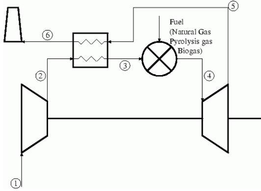
Figure 1. Flowsheet of a recuperated gas turbine
