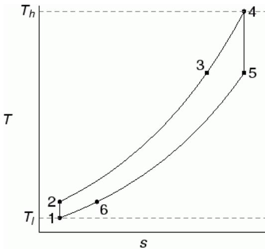
Figure 2. T-s-diagram for the recuperated gas turbine cycle
