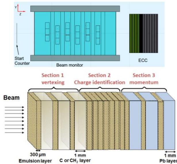
Figure 1. The nuclear emulsion cloud chamber setup. Top: the complete experimental setup with the start counter, the beam monitor and the ECC detectors. Bottom: ECC sections.
