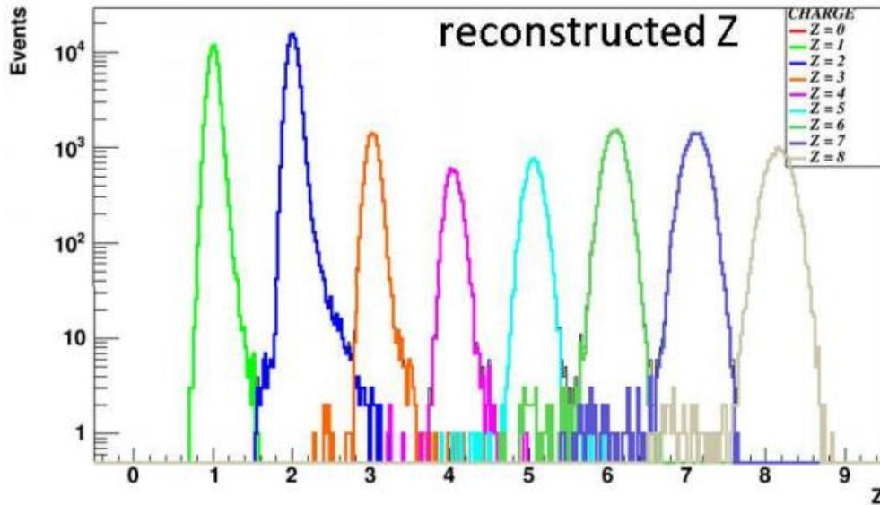
Figure 3. Charge reconstruction distribution for fragments produced by  $^{16}\text{O}$  beam at 220 MeV/u on a target of  $\text{C}_2\text{H}_4$ , (FLUKA simulation)
