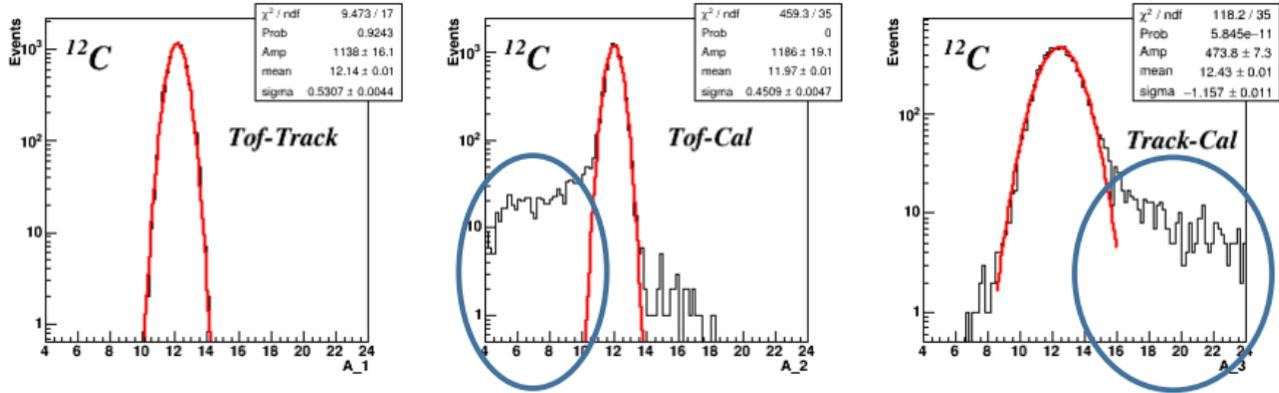
Figure 4.  $A_1$ ,  $A_2$  and  $A_3$  mass reconstruction distributions for carbon ion produced by  $^{16}\text{O}$  beam at 200 MeV/u on  $\text{C}_2\text{H}_4$  target, by means of FLUKA simulation. The two blobs in the second and third plots point out the distribution tails given by the loss of energy measurement of the neutrons in the calorimeter.
