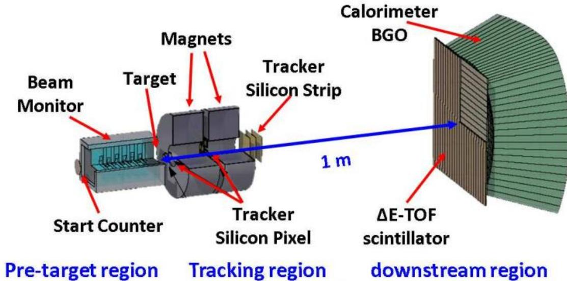
Figure 2. The FOOT electronic experimental setup
