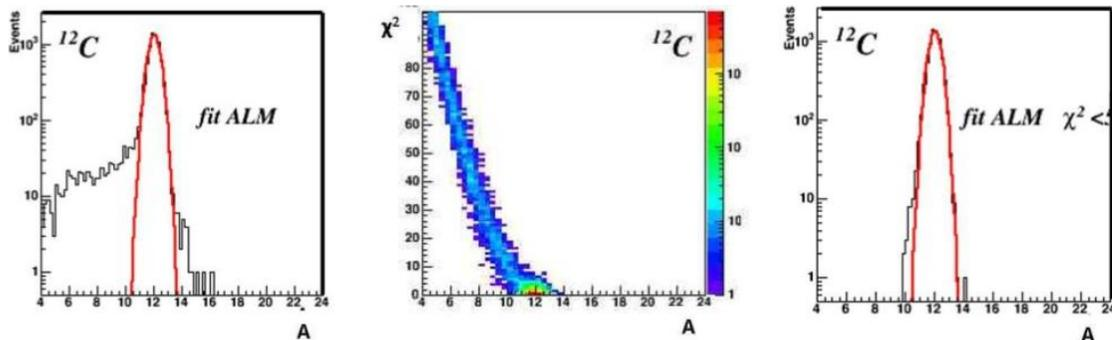
Figure 5. Mass identification with the  $\chi^2$  and the ALM method for carbon ion produced by  $^{16}\text{O}$  beam at 200 MeV/u on  $\text{C}_2\text{H}_4$  target, by means of FLUKA simulation. From left to right: the first plot is the mass reconstruction performed with ALM method; the second plot is the mass calculated with the  $\chi^2$  technique; the last plot is the final mass reconstruction with the ALM method and  $\chi^2 < 5$
