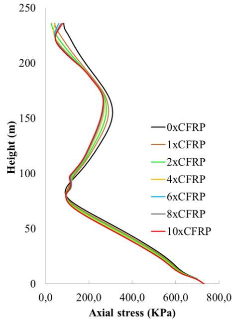
Figure 8. The change of the stress amount in the tower shell in the height of the tower
