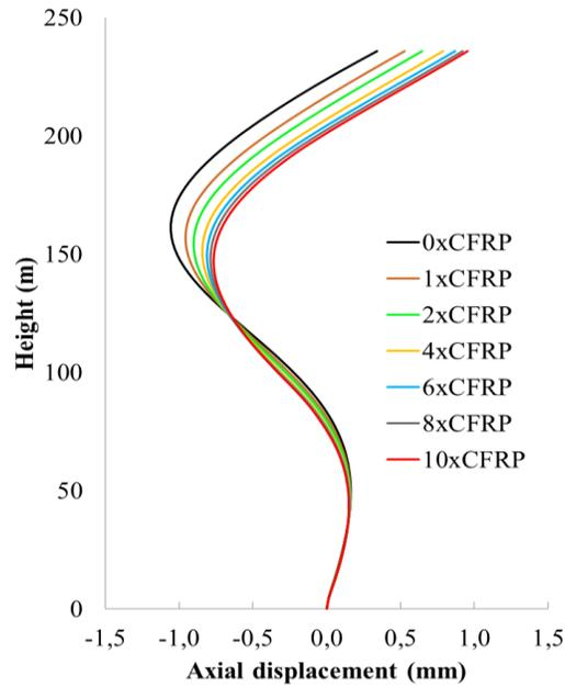
Figure 6. The change of the displacement amount in the tower shell in the height of the tower
