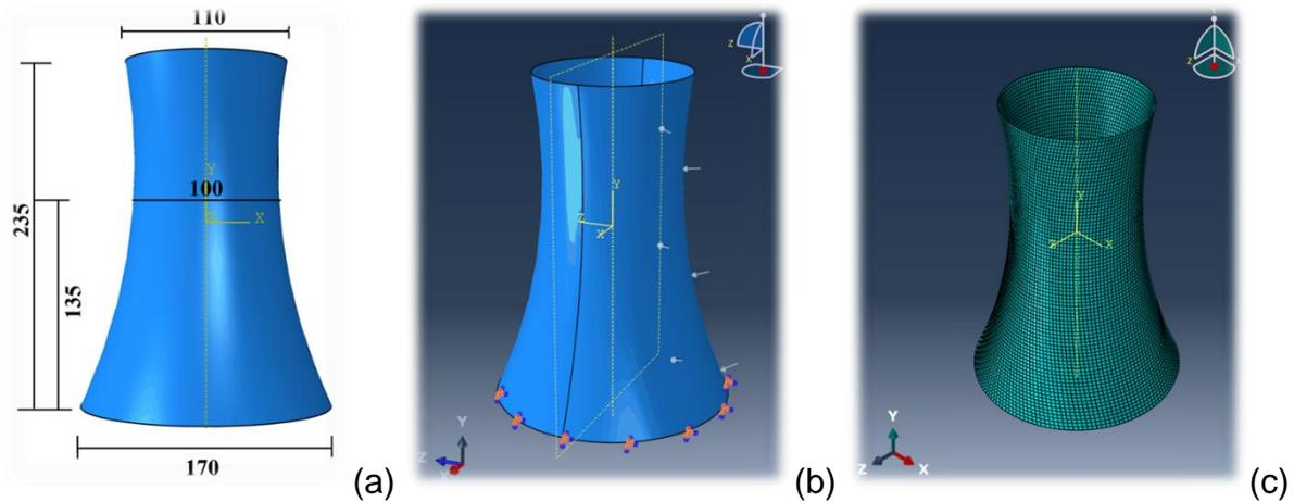
Figure 3. Dimensions (a), boundary conditions (b) and typical mesh appearance of cooling tower.
