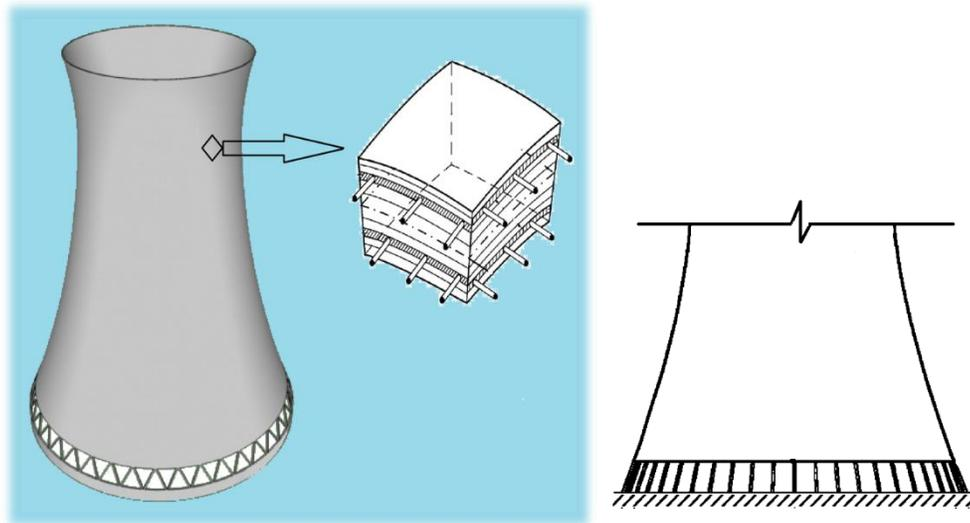
Figure 2. A schematic image of the structure element detail (left) and column connections (right) of cooling tower.
