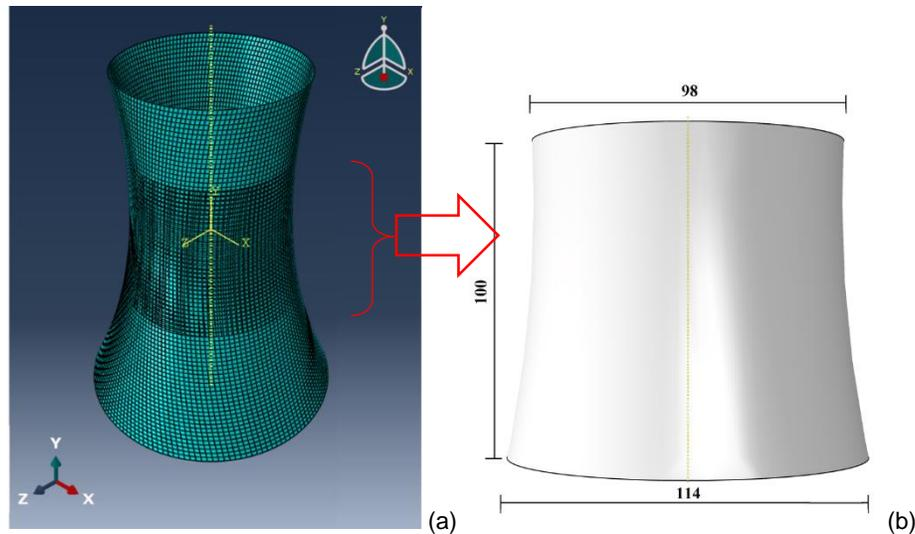
Figure 4. Typical mesh appearance (a), and dimensions (b) of the CFRP.
