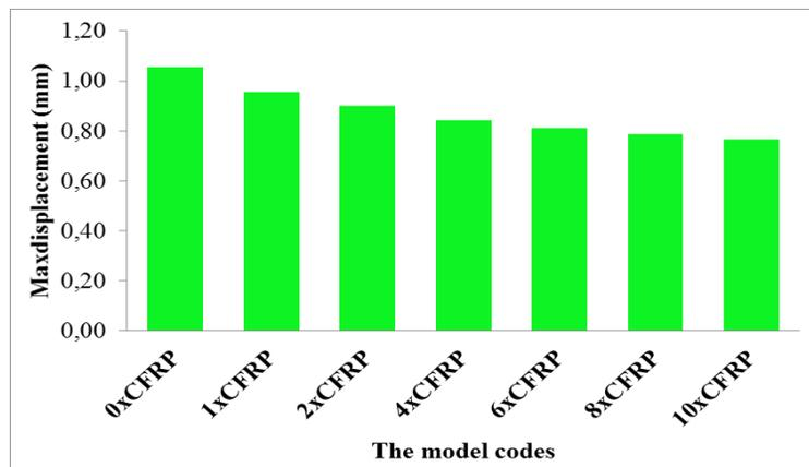
Figure 7. Maximum displacement values with CFRP thickness
