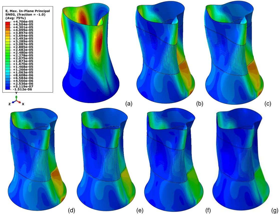
Figure 5. Deformation Contours of unreinforced and layer CFRP reinforced tower; (a); unreinforced, (b); 1xCFRP, (c); 2xCFRP, (d); 4xCFRP, (e); 6xCFRP, (f); 8xCFRP and (g); 10xCFRP reinforced.
