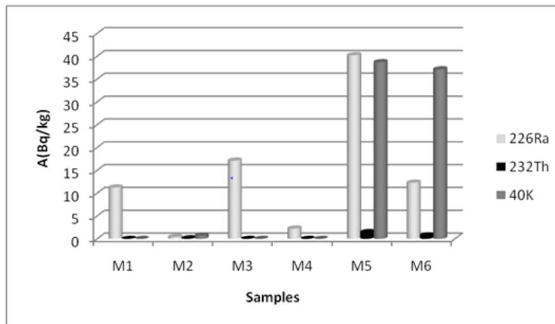
FIG. 2. Activity concentrations of  $^{226}\text{Ra}$ ,  $^{232}\text{Th}$  and  $^{40}\text{K}$  for the investigated samples.
