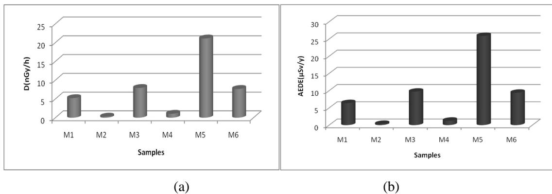
FIG.3. (a) Absorbed dose rate in air and (b) Annual effective dose equivalent for the studied samples.
