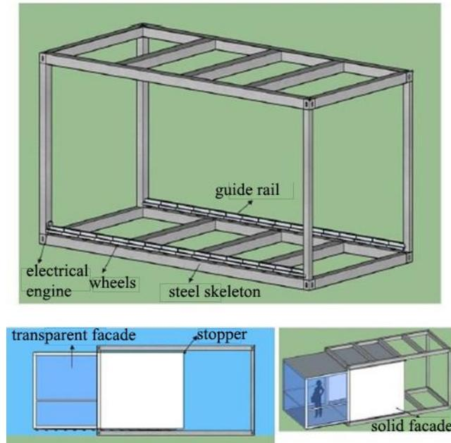
**Figure 13.** Cell sliding system construction drawings [22]
