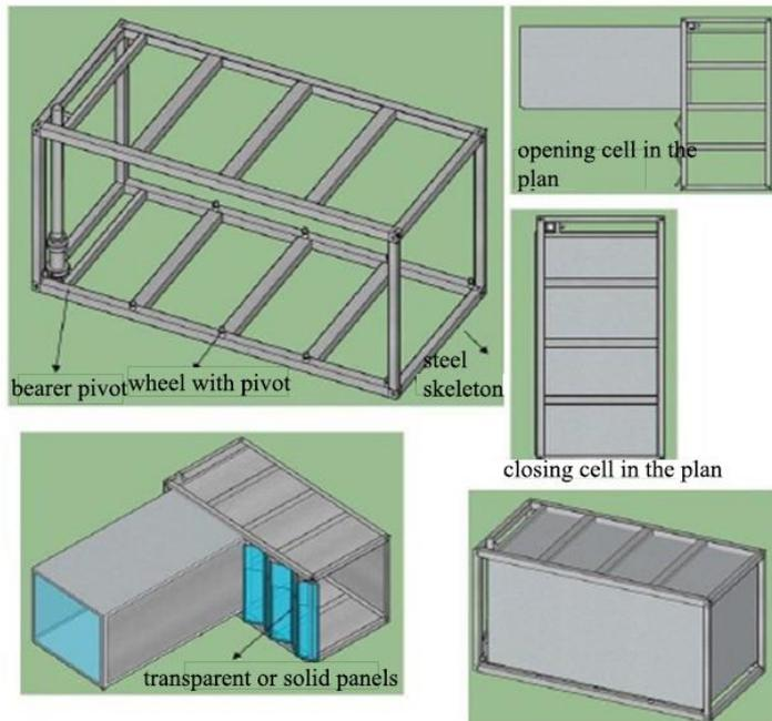
**Figure 14.** Pivoted cell system construction drawings [22]
