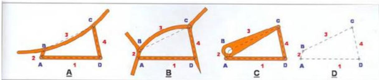
**Figure 1.** The simplest plane mechanism samples consisting of four bars [4]
