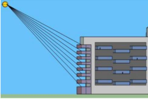
**Figure 33.** Perspective of point block in getting light with kinetic systems before opening [22]
