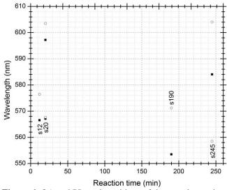
**Figure 6.** OA and PL peak positions of the samples against the reaction time. OA and PL peak wavelengths are shown with filled squares ( $\blacksquare$ ) and open circles ( $\circ$ ), respectively.
