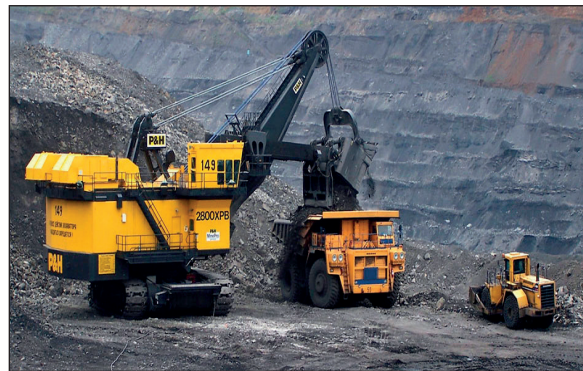
Photograph 1. Dump segment of cycle time of a 35 m 3 electric rope shovel (Anon (b), 2015)
