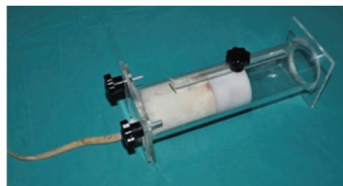
Figure 1. An overview of the application of immobilization stress by the transparent plexiglass apparatus.
