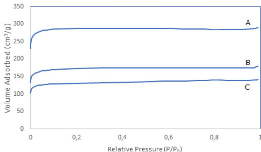
**Figure 2:** Adsorption isotherms of N<sub>2</sub> **A.** Activated carbon sample at 600 °C 100 mL / min N<sub>2</sub> carbonization and at 800°C with 100 mL / min CO<sub>2</sub> activation **B.** Activated carbon sample at 800 °C 100 mL / min N<sub>2</sub> carbonization and at 900 °C with 100 mL / min CO<sub>2</sub> activation. **C.** Activated carbon sample at 300 °C 100 mL / min N<sub>2</sub> carbonization and at 800 °C with 100 mL / min CO<sub>2</sub> activation.
