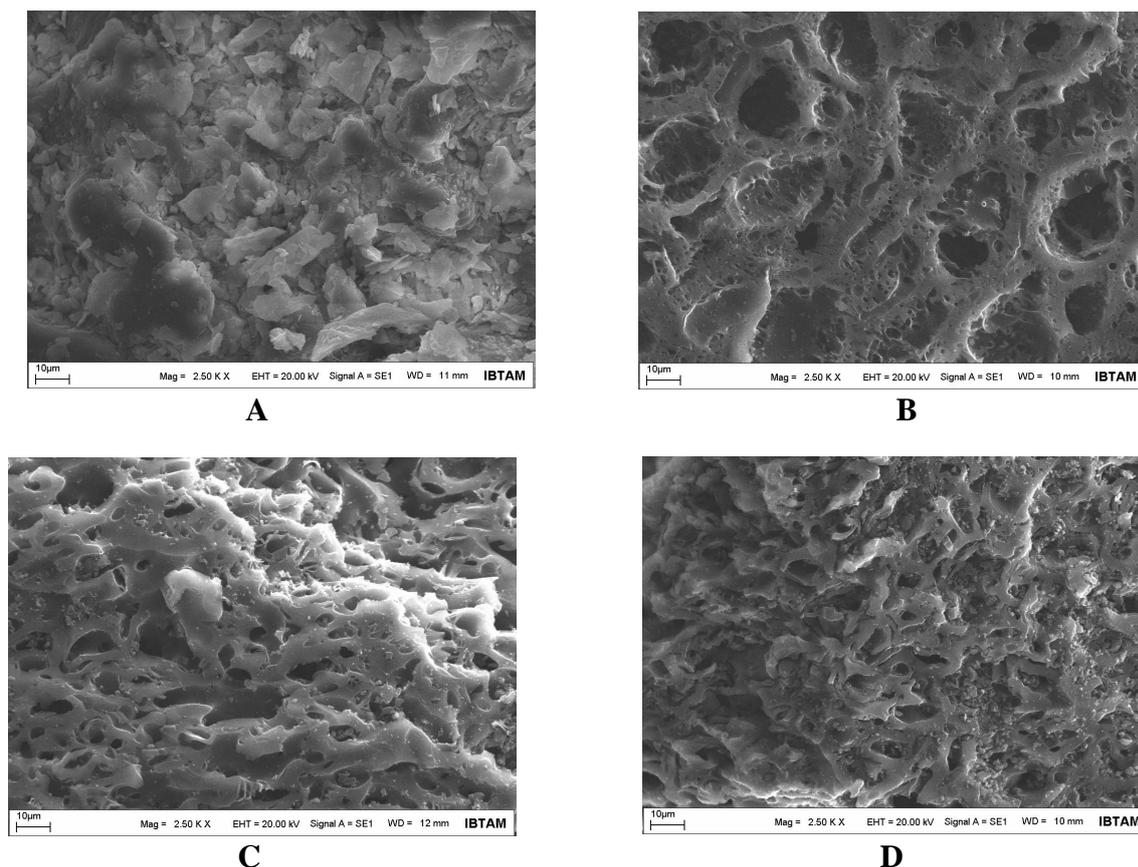
**Figure 4:** **A.** SEM image of raw pistachio shell **B.** Activated carbon sample at 600 °C 100 ml / min N<sub>2</sub> carbonization and at 800 °C with 100 mL / min CO<sub>2</sub> activation **C** Activated carbon sample at 500 °C 100 mL / min N<sub>2</sub> carbonization and at 800 °C with 100 mL / min CO<sub>2</sub> activation **D.** Activated carbon sample at 300 °C 100 mL / min N<sub>2</sub> carbonization and at 800 °C with 100 mL / min CO<sub>2</sub> activation.
