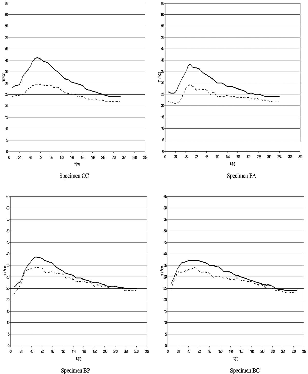
Fig. 4. Concrete Temperature ( — middle, - - - surface)
