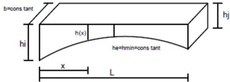
**Figure 1.** Variable cross-sectioned element
