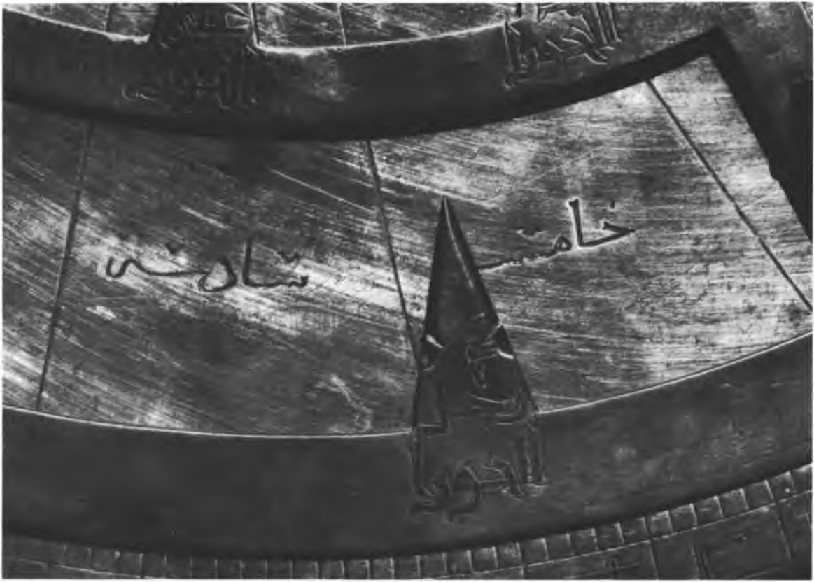
3a The pointer for rijl al-jawzā' above the hour-curves of a plate.
