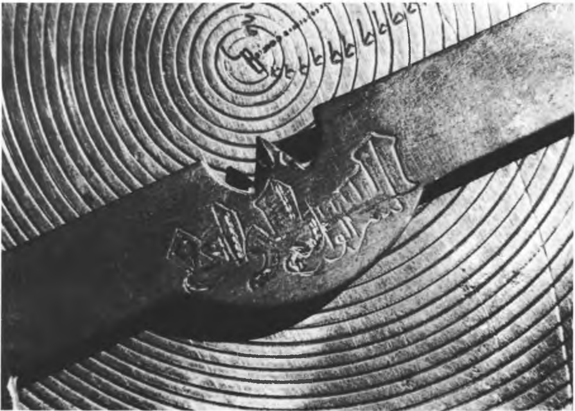
3b The pointer for al-nasr al-wāqi' above the altitude circles around the zenith of one of the plates.
