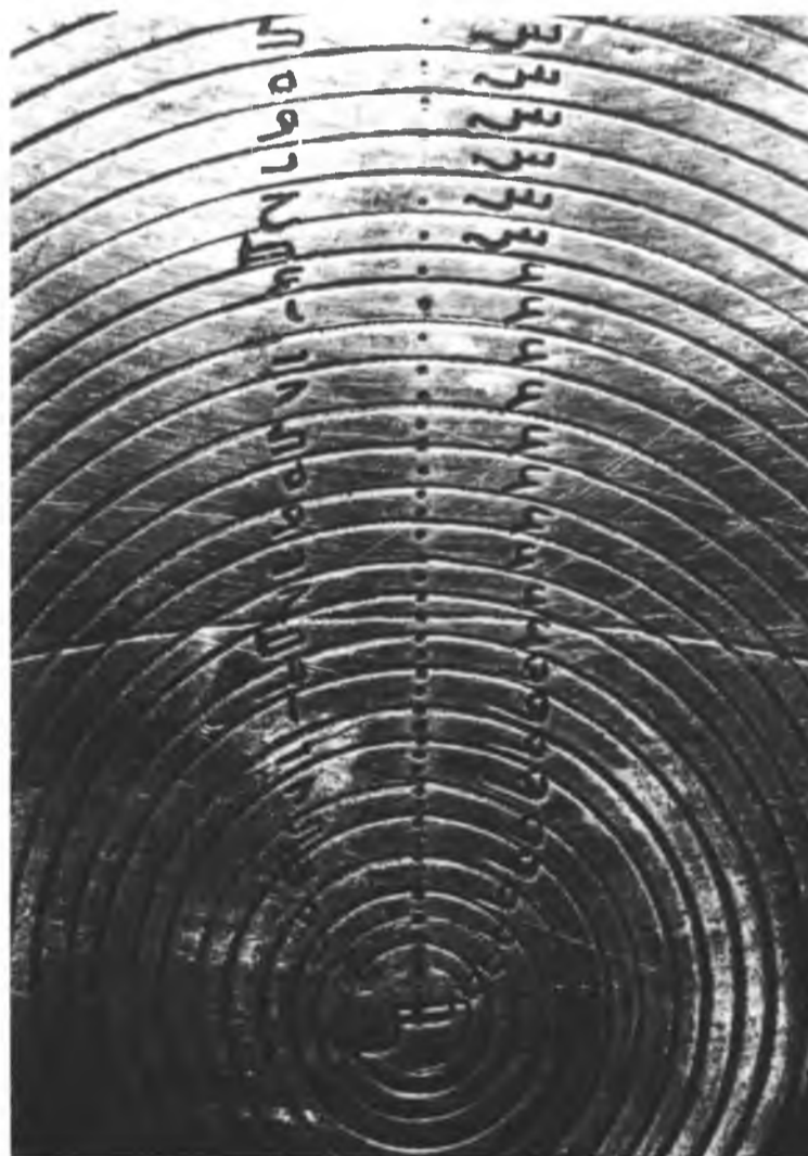
4b The meridian scale on the plate for atitude 35°.
