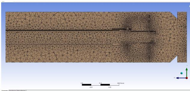
Figure 8. Mesh details of the NG-2 burner part
