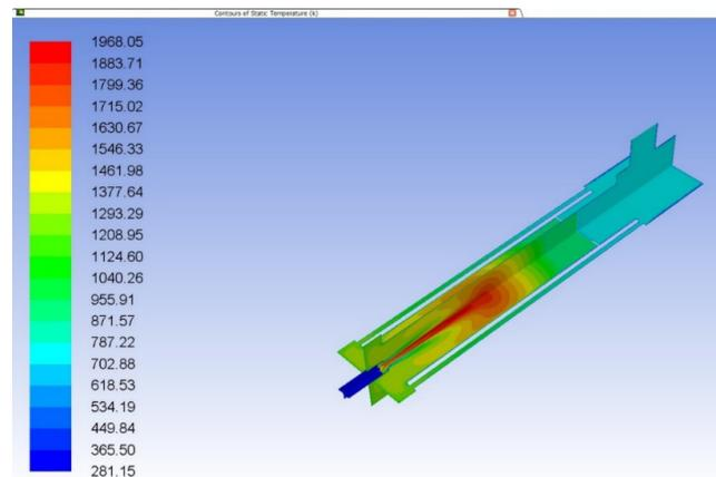
Figure 9. Temperature [K] contour plot of the NG-2
