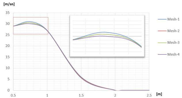
Figure 2. Axial velocity distribution in axial direction. [m]
