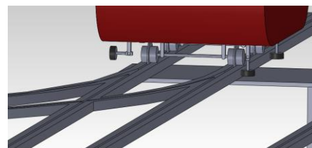
Figure 5. Channelling part and wheels, channelling left, front bottom view.
