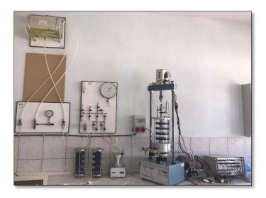
Figure 5. Dynamic triaxial test system
