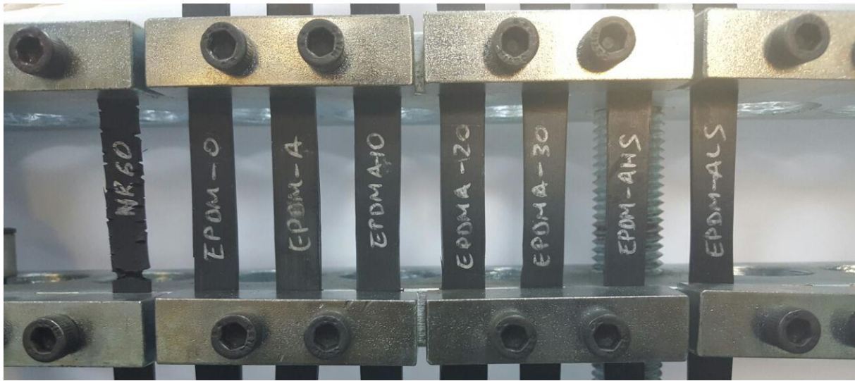
Figure 2. Vulcanizate samples after ozone aging
