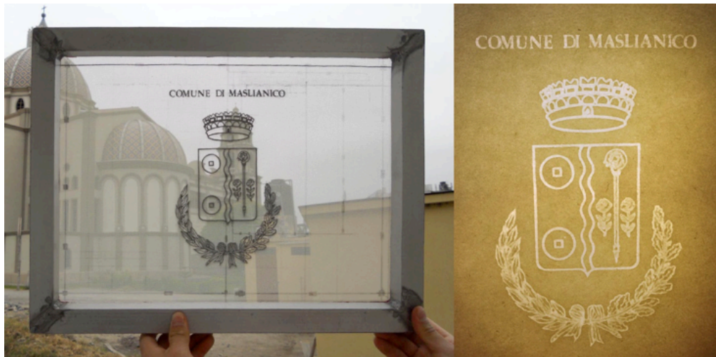
Visual 3. Left: The moulded mesh used to produce the paper with the watermark. Right: The watermark can be observed when paper is looked at in front of a light source. (Source: http://www.cartamaanonelleande.org/IT/galleria_filigrane )
