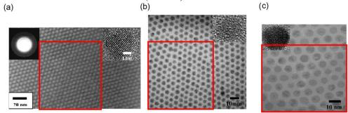
**Figure 1.** TEM images of arrays of a) 3.5 nm, b) 5 nm and c) 7 nm palladium nanoparticles synthesized by Sang-Wook Kim and coworkers.
