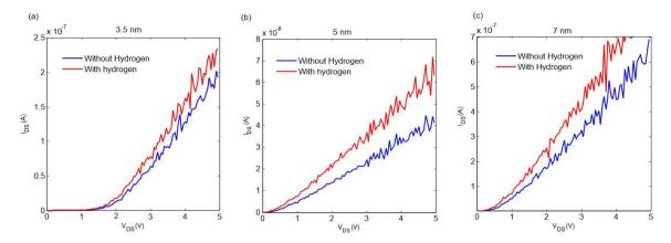
**Figure 4.** Effect of hydrogen gas on the IV characteristics of selected sections of arrays for a) 3.5 nm, b) 5 nm and c) 7 nm nano-islands.
