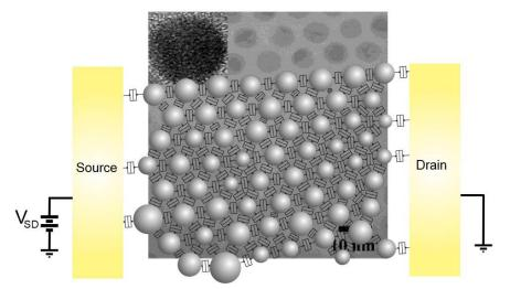
Figure 2. Schematic diagram of equivalent circuits consisting palladium nano-islands and tunneling junctions.
