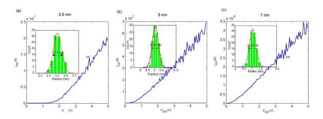
Figure 3. IV characteristics of selected sections of arrays for a) 3.5 nm, b) 5 nm and c) 7 nm nano-islands.
