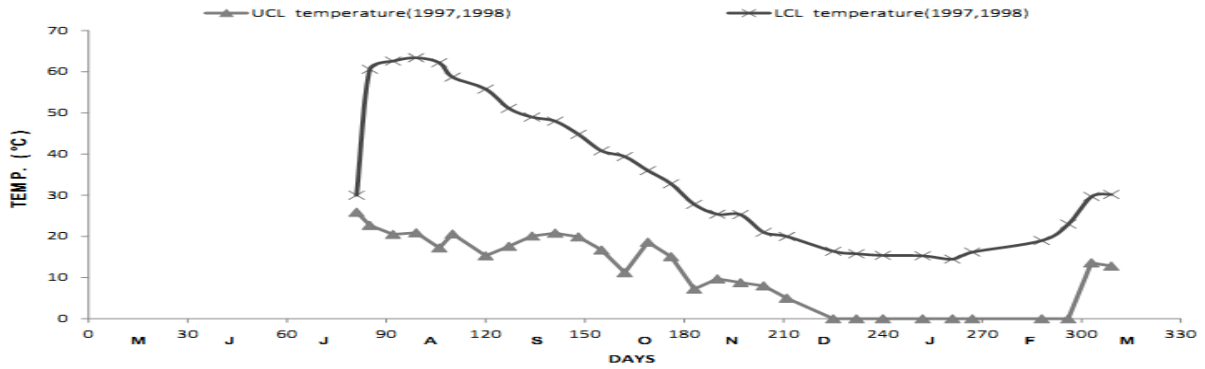
Figure 2. Time variations of the temperature in the upper and lower convective layers
