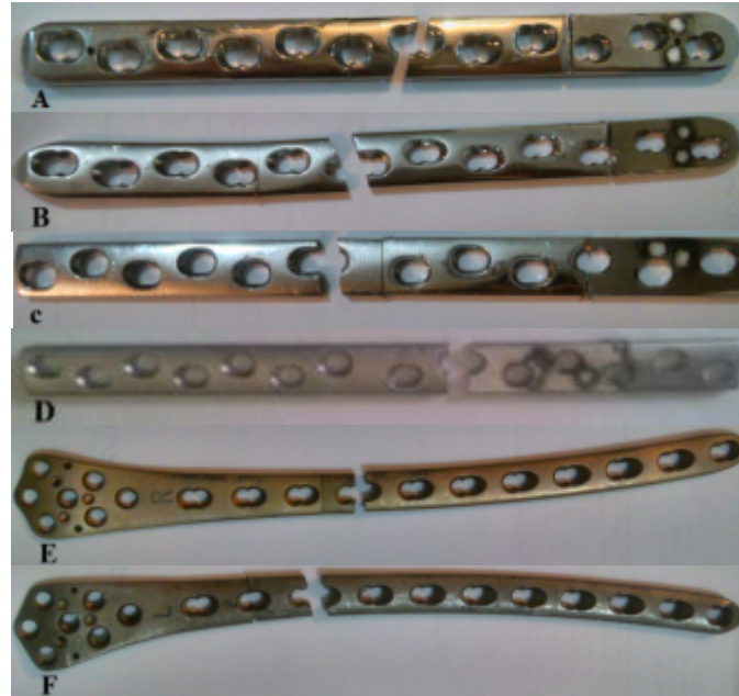
Figure 1. Six investigated plates with cut parts for SEM analysis of failure surface; samples A) 1, B) 2, C) 3, D) 4, E) 5 and F) 6.
