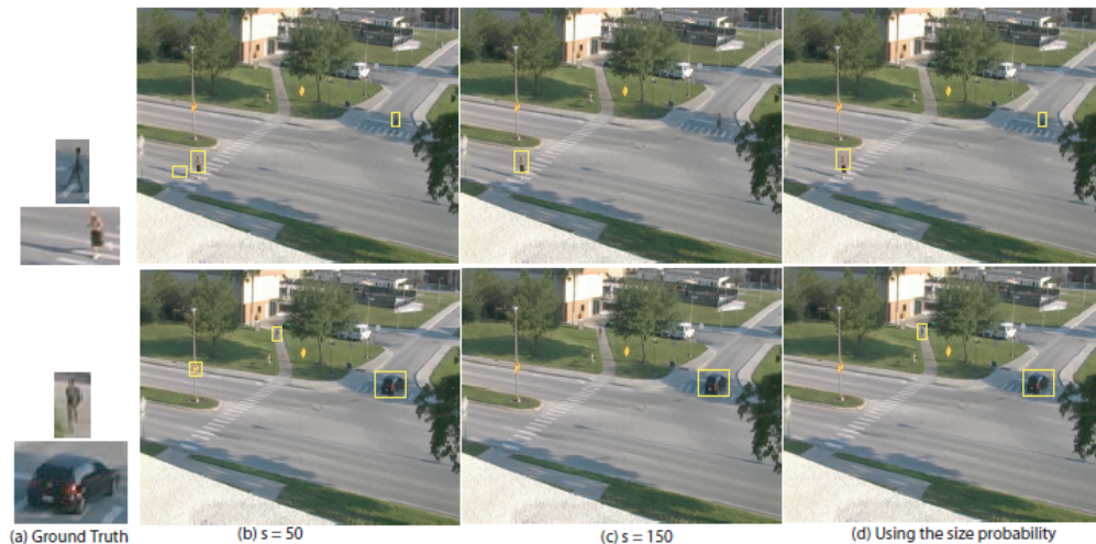
Figure 6. Scene 2. Improvement in object detection by the proposed size model. Each row presents an instance in the same video. Column (a) shows the manually extracted patches of the objects currently present in the scene. Column (b) is the output when a uniform global value of s = 50 is used. Noisy foreground blobs are also detected as valid objects (red ellipses). (c) presents output when s = 150 is used throughout the scene. Individuals are not detected (red ellipses) when the object size is small. (d) presents results of the proposed size model. In both scenarios the valid objects are detected and the noisy observations are avoided.
