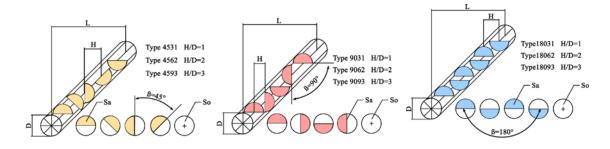
Figure 2: Schematics of half circle baffled tubes
