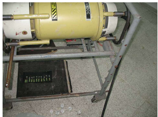
Figure 5. Film, penetrometer, stenciling pattern and setting the beam
