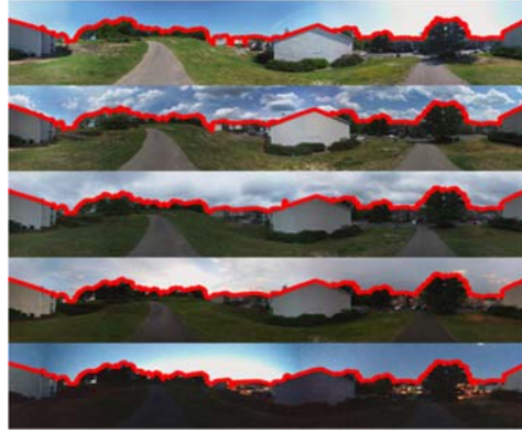
Figure A. Skylines found on photos that are taken from the same spot at different times
