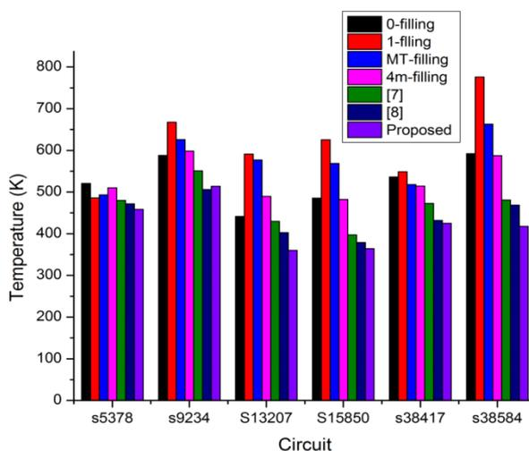
**Figure 3.** Peak temperature for different X-filling
