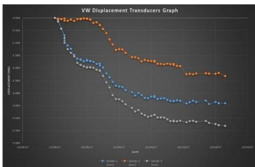
Figure 11. Deformation graphs obtained by Extensometer-1 data
