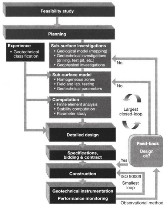
Figure 9. Flow-process Diagram.
