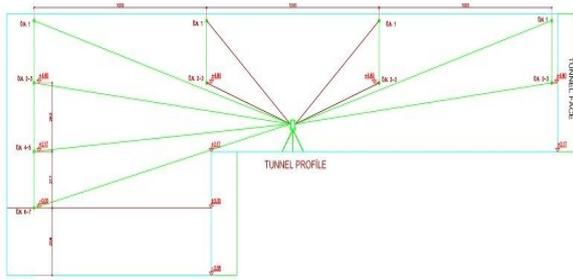
Figure 4. Tunnel deformation survey method
