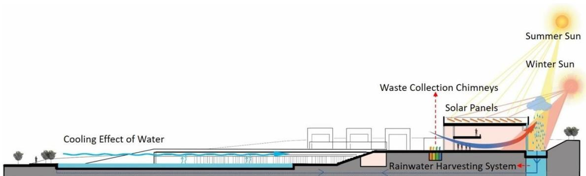
Fig. 4. Design Decisions from an Ecological Perspective in Section III-III
