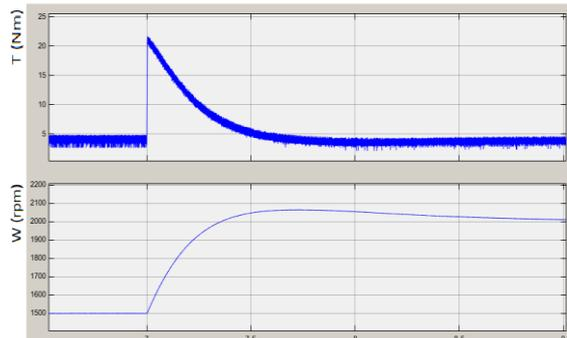
**Figure 8.** Speed reference impact, 4Nm at 2800 rpm.
