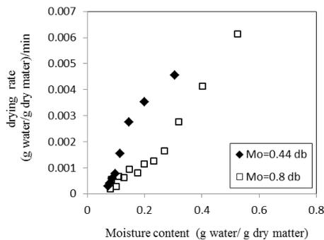
Figure 6. Effect of the initial moisture content on spouted bed drying of rosehip and variation of the drying rate for 0.44 and 0.8 initial moisture contents.
