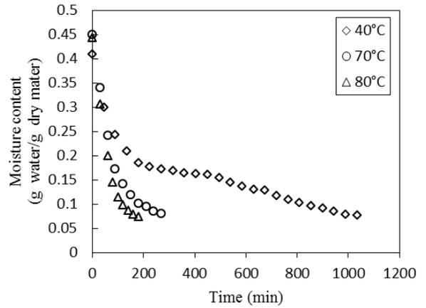
**Figure 3.** The spouted bed drying curve of rosehip.
