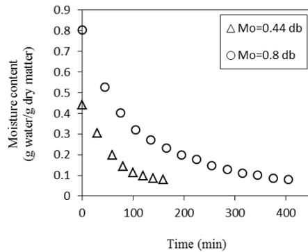
Figure 5. Effect of the initial moisture content on spouted bed drying of rosehip and variation of the drying rate for 0.44 and 0.8 initial moisture contents.
