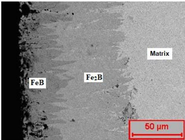
Figure 4. SEM (BE) image of boronized 34CrAlNi7
