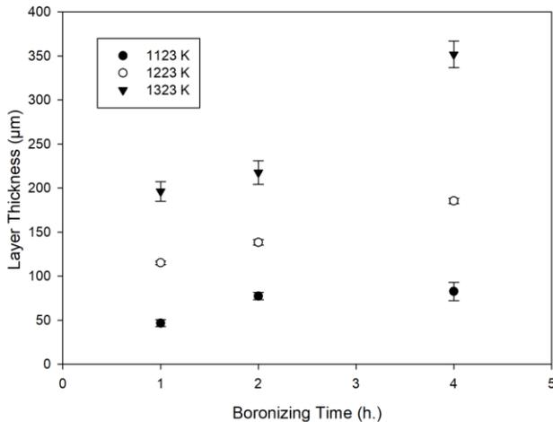
Figure 5. Thicknesses of boride layer on 34CrAlNi7
