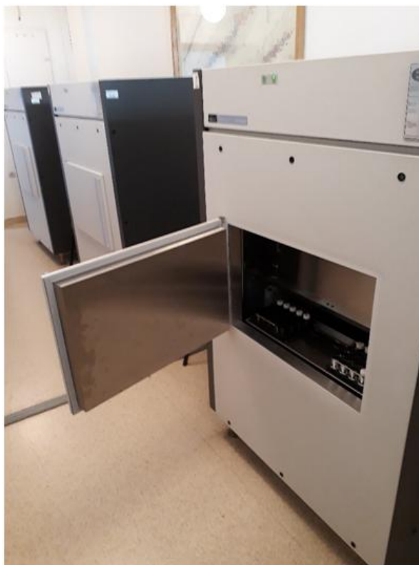
Figure 2. Perkin Elmer Quantulus1220 liquid scintillation counting device.
