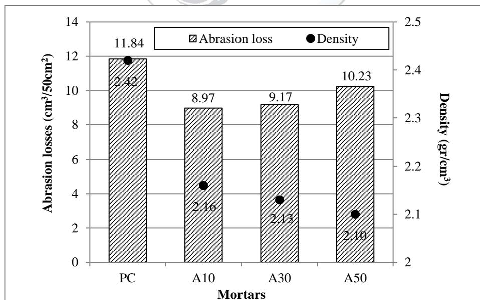
Figure 4. Abrasion loss and density variation for mortar
