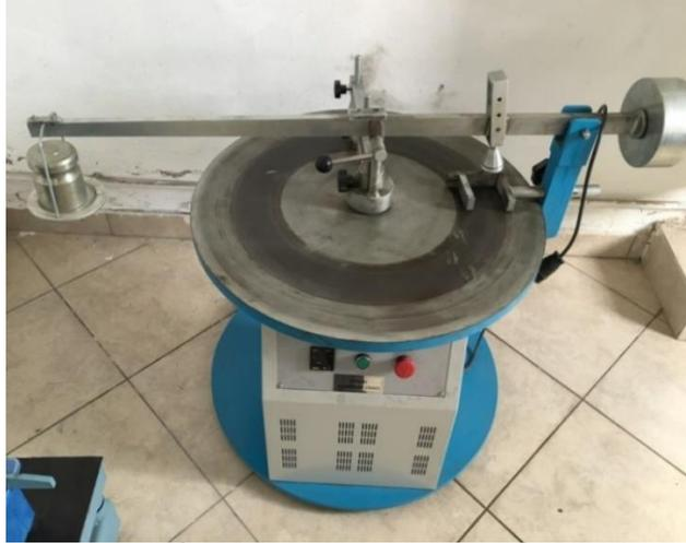
Figure 1. Bohme abrasion test device
