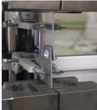
Figure 5. Zwick Z010 lap-shear tensile tests machine.
