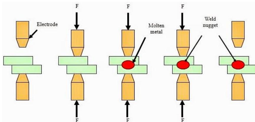
Figure 1. A schematic presentation of the ERSW process [5].
