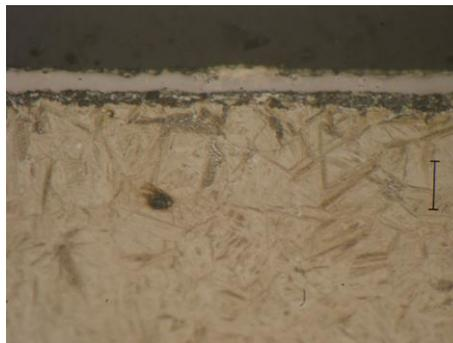
Figure 5. Optical micrograph showing the surface of the interstitial-free steel first titanium diffused at 1000 °C for 2 hours and then boronized at 900 °C for 45 min by applying a current density of 0.10 A/cm<sup>2</sup> (Scale length: 10 µm)
