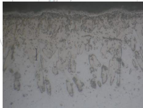
*Figure 7. Optical micrograph of the surface of the interstitial-free steel titanium diffused at 1000 °C for 2 hours and then boronized at 900 °C for 120 min by applying a current density of 0.40  $\text{A}/\text{cm}^2$  (Scale length: 10  $\mu\text{m}$ )*
