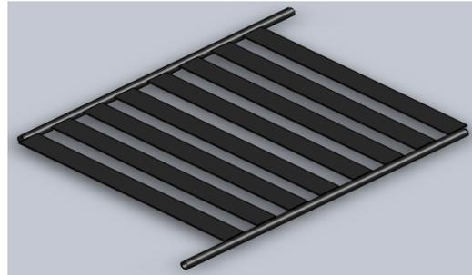
Figure 3. Developed plate heat exchanger
