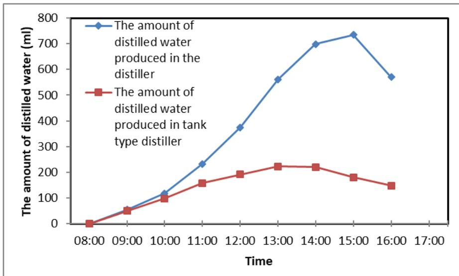
Figure 11. Amounts of basin-type and tank-type distiller produced in solar supported integrated water heating-distillation system
