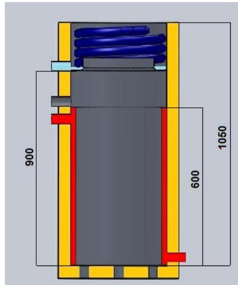
Figure 4. Dimensions of tank-type distiller (mm)
