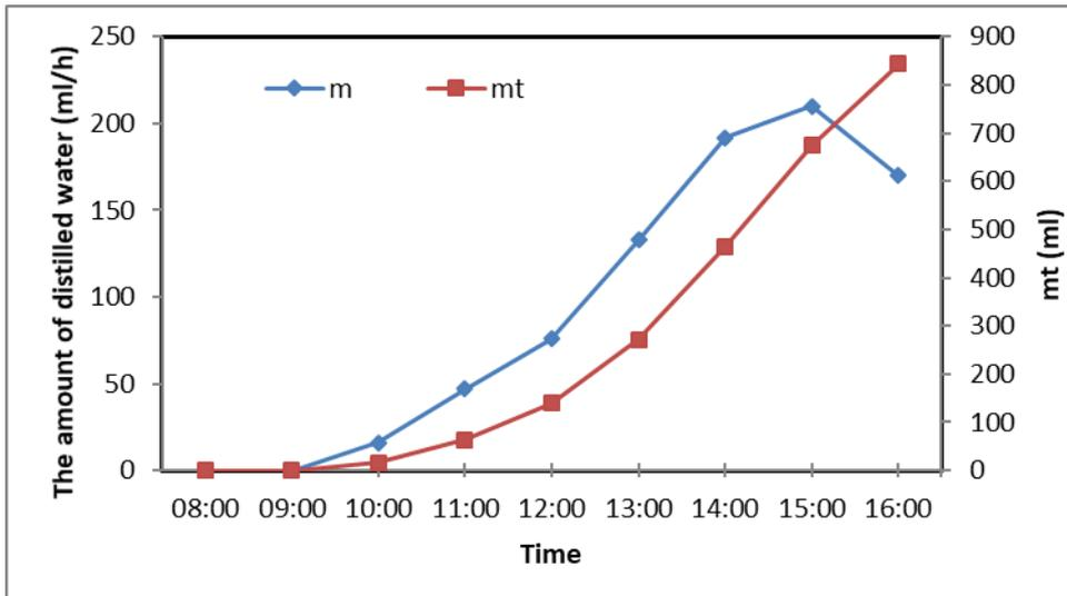
Figure 9. Hourly and total amount of water produced for conventional basin-type distiller
