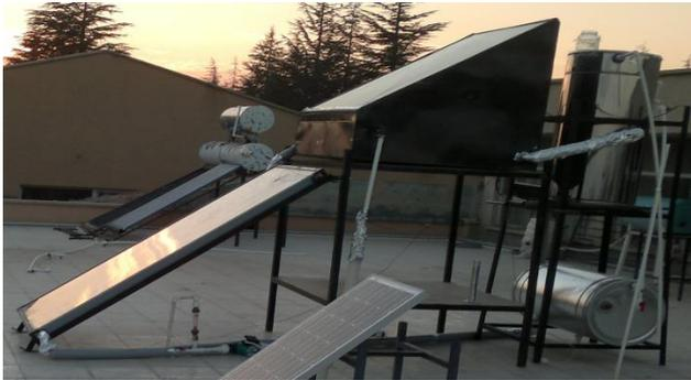
Figure 2. Photo of distiller system integrated with hot water collector
