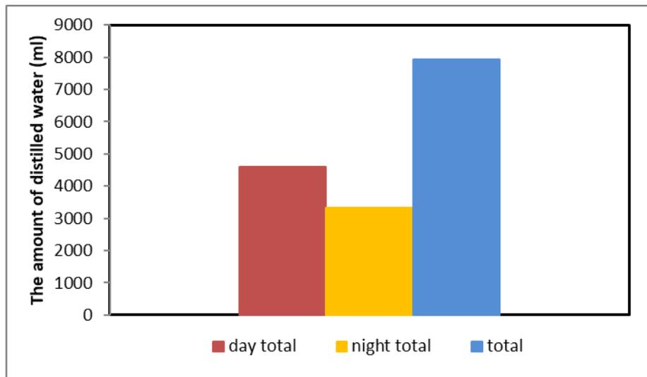
**Figure 13.** Daytime, night-time and total amount of water produced solar supported integrated water heating-distillation system
