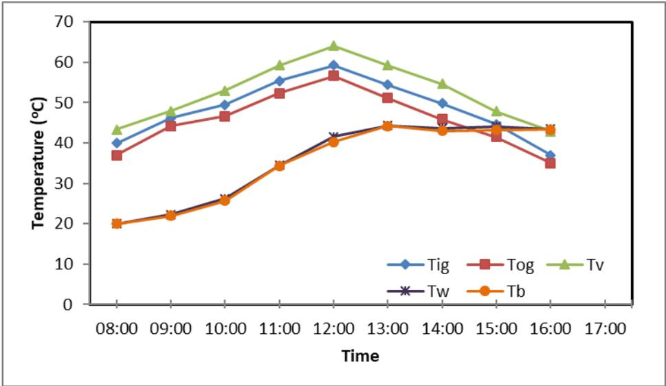
Figure 7. Temperature changes in conventional basin-type distiller
