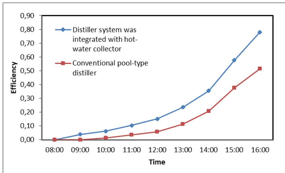
**Figure 14.** Efficiencies of solar supported integrated water heating-distillation system and conventional basin type
