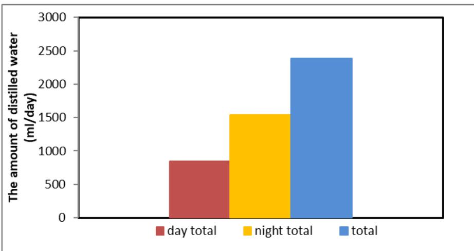
Figure 12. Daytime, night-time and total amount of water produced for conventional basin-type distiller
