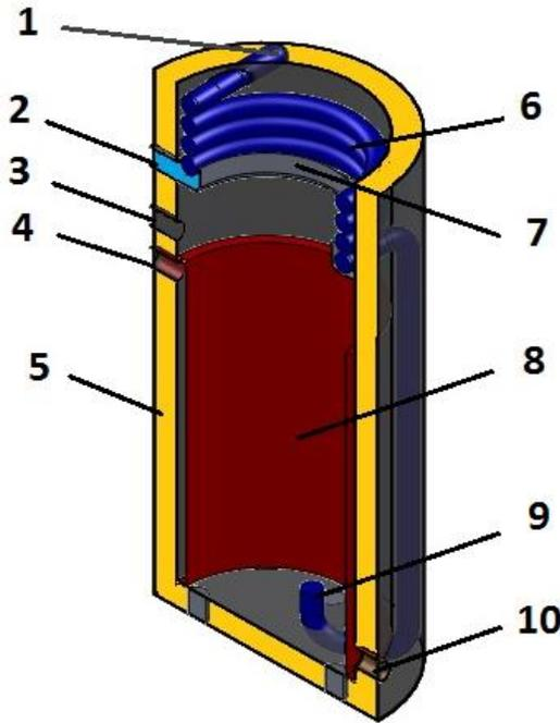
**Figure 5.** Distillation tank. (1. Tap water inlet 2. fresh water outlet, 3. Hot water exit, 4. Hot water inlet, 5. Glass wool, 6. Upper serpentine, 7. Fresh water collection pipe, 8. Lower serpentine, 9. Cold water inlet, 10. Hot water exit.)
