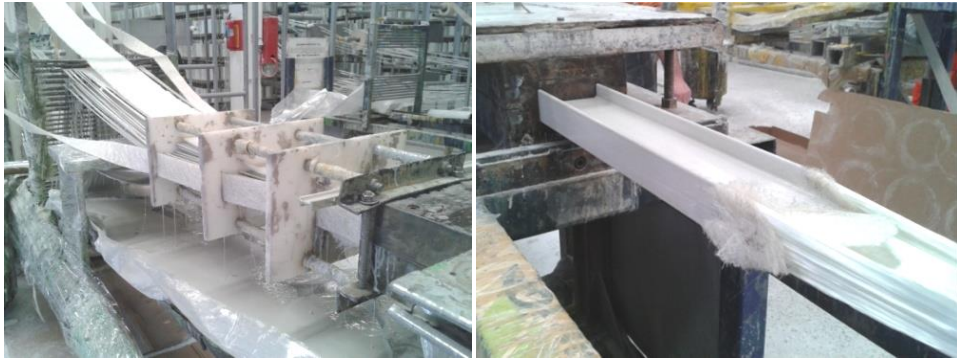
Fig. 1 Pultrusion line and manufacturing process of the composite profiles.
