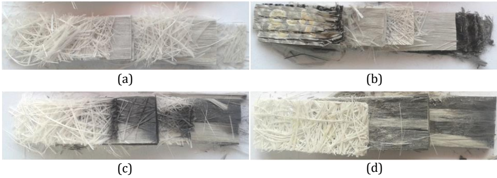
Fig. 6 Photos of calcinated specimens and their reinforcement configurations (a) Type 1 specimen, (b) Type 2 specimen, (c) Type 3 specimen and (d) Type 4 specimen.
