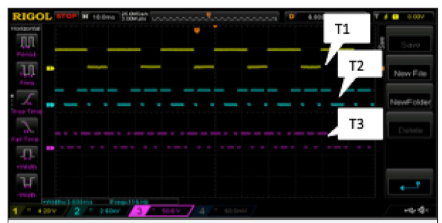
Figure 22. Switching signals of PUC-7 level on DSO
