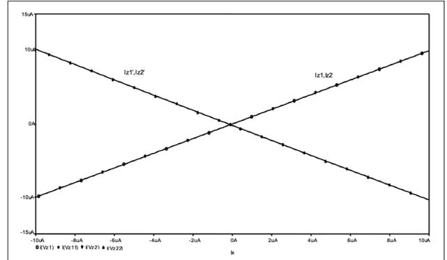
Figure 9. FGMOS UCCII DC current transfer characteristics
