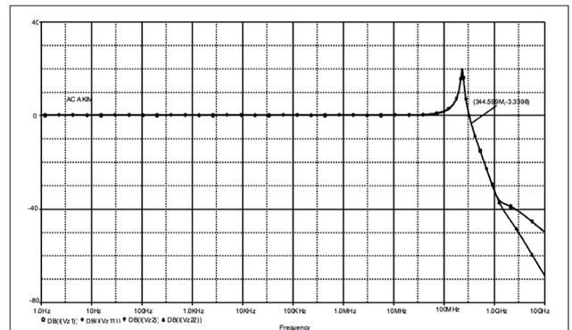
Figure 11. FGMOS FDCII AC current transfer characteristics ( $I_X-I_{Z1,2,12'}$ )
