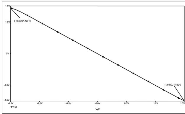
Figure 7. FGMOS UCCII DC voltage transfer characteristics ( $V_X-V_{Y2}$ )
