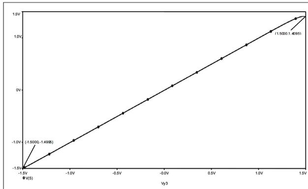
Figure 8. FGMOS UCCII DC voltage transfer characteristics ( $V_X-V_{Y3}$ )
