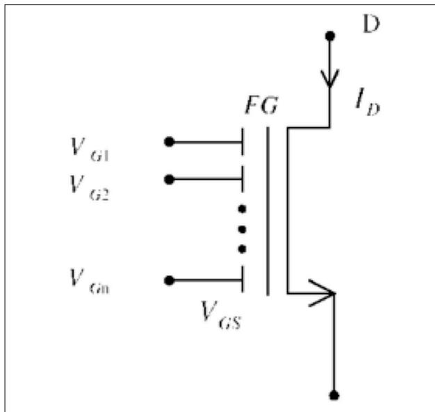
Figure 1. Diagram of a n-input n-channel FGMOS transistor
