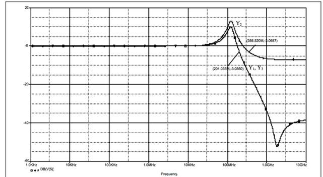
Figure 10. FGMOS UCCII AC voltage transfer characteristics ( $V_X-V_{Y1,2,3}$ )
