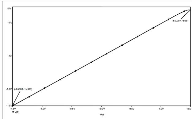
Figure 6. FGMOS UCCII DC voltage transfer characteristics ( $V_X-V_{Y1}$ )
