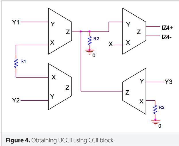
Figure 4. Obtaining UCCII using CCII block
