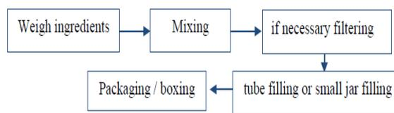
**Figure 6.** Semi-solid form drug production flowchart [89].
