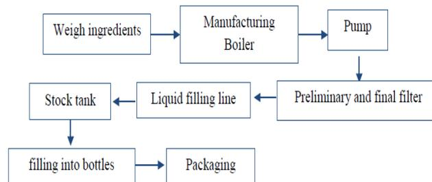
**Figure 7.** Liquid form drug production flowchart [89].
