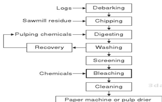
Figure 2. Pulp and Paper production process flow chart [66].
