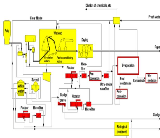
**Figure 3.** Toolbox for possible internal treatment and reuse of paper machine waters [87].
