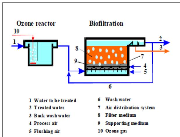
**Figure 4.** Combined process of ozonation and fixed bed biofilm reactors [70].
