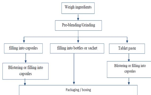
**Figure 5.** Tablet manufacturing process flow diagram [89].
