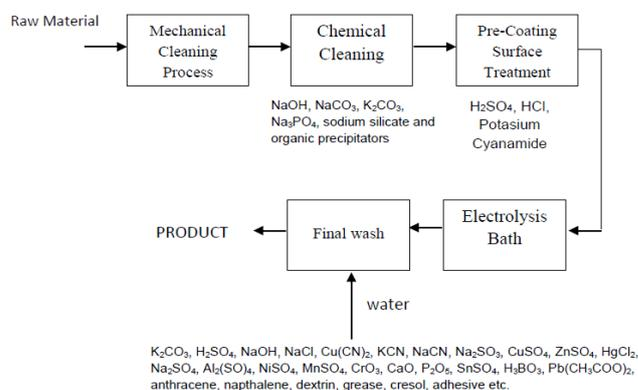
Figure 1. General flow diagram of the coating process [26].
